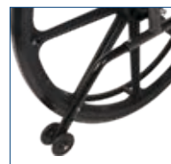
Adjustable anti-tippers with push-pin flip-up wheels
