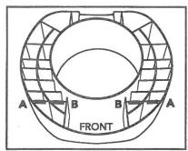
4 Slip the enclosed tabs onto the bottom framework making sure they come in contact with the surface of the toilet rim by using outer position A or inner position B
