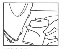
2 Slide the locking plate between the toilet and the toilet seat 3 Firmly tighten the toilet seat screws
