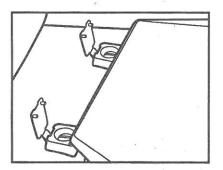
1 Use a screw driver to loosen the toilet seat screws – you do not need to completely remove the screws
