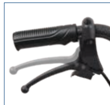
Companion activated hand brakes
